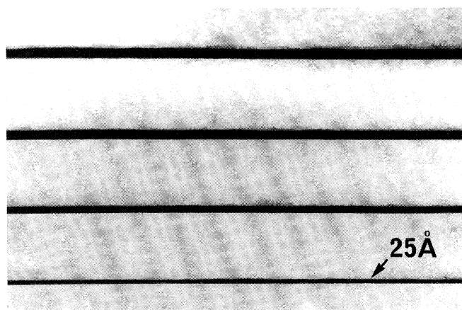
Figure 1. TEM cross-sectional image, bright-field, 200 reflection, of InGaAs quantum wells (dark) in InP. (After Cullis 1990.)
